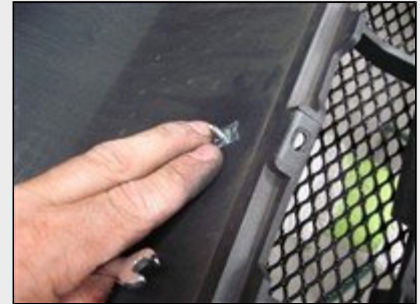
Picture #30: Fasten vent grille in place using supplied hardware.
