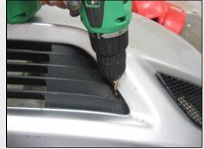
Picture #27: Drill slotted hole in plastic for the mounting tab.
