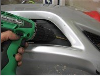
Picture #25: Drill 3/16 inch hole for the grille mounting screws.
