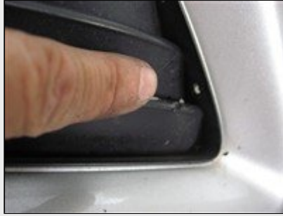
Picture #26: If you dont want to cut the factory grille center out you will need to drill a small slotted hole in order for the grille tab to sit flush with the mounting clip installed.
