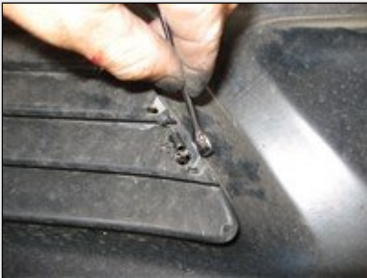
Picture #31: Fasten Grille in place with the supplied hardware.
